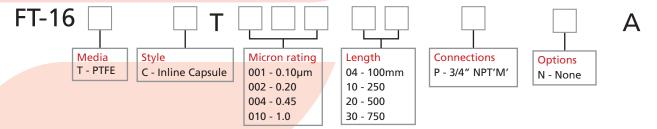
Example: 16TCT002-20PNA = PTFE media, inline capsule, 0.2µm, double length 20" long, 3/4" NPT'M' connections, same side vent alignment.
