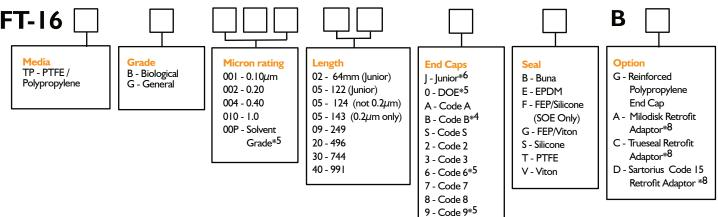
Example: 16TPB002-203FA = PTFE media with polypropylene core, Biological Grade, 0.02μm, double length 20" long, Code 3 end fitting with FEP/Silicone seal.
