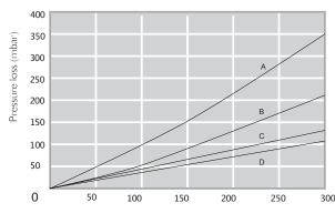
Air Flow Rates (m3/hr @ 0barg) A=0.2μm B=0.4μm C=0.5/0.6μm D=1.0μm+
